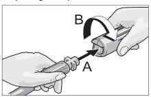
**Step 1** Install the High/Low pressure nozzle. Set the nozzle to the low pressure setting by turning the nozzle collar. The nozzle must be set in the low pressure position to apply detergents.
